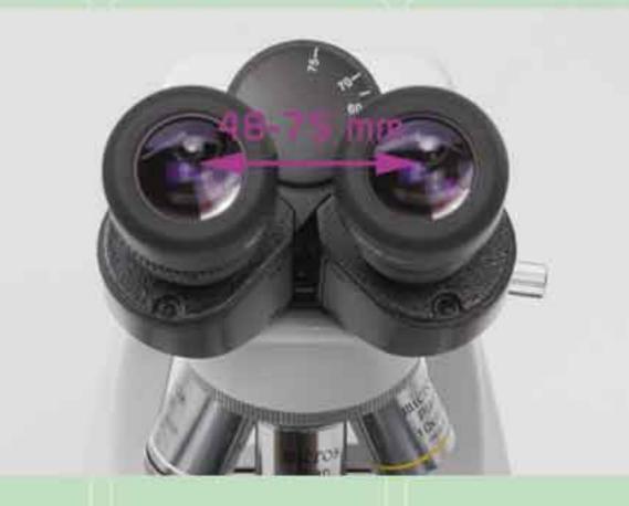
With the ARCTYPE tube the eyepieces can be positioned in two different heights. The eyepoint adjustment range is 350 – 395 mm, which means small and tall users can have an ergonomic and relaxed posture while observing. The interpupillary distance adjustment (48 – 75 mm) and the diopter adjustment ensure that the microscope easily fits to every user.
