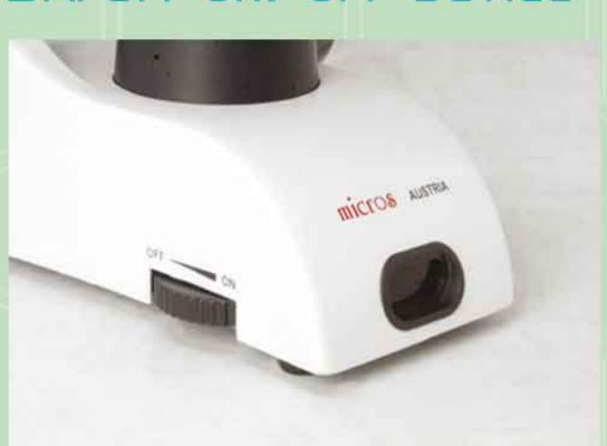
The power switch is combined with the brightness adjustment for protecting the eyes. In order to turn the device off, the brightness adjustment has to be on the lowest position. With the safety rotary control device no harm can come to the eyes of too bright light at full power while turning on the microscope.
